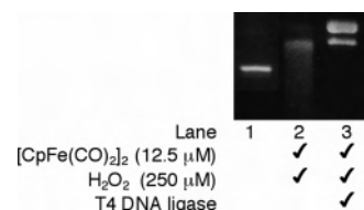
Figure 5. Religation studies of the cleavage of pBR322 DNA (30 μM/bp in 10% THF/water) by 2 and H 2 O 2 . Samples were incubated under ambient light for 30 min. After concentration and removal of 2 by ultrafiltration, an aliquot of the sample in lane 2 was treated with T4 DNA ligase (lane 3).
